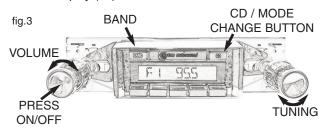
3. Depress the CD button (4) to toggle the functions of the radio .The sequence displayed will be: Radio-USB-CDC-AUX-Radio.
