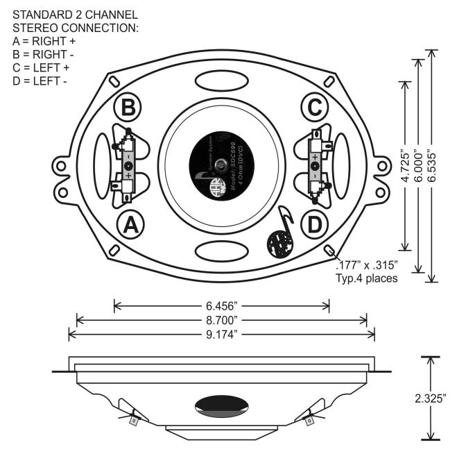
TO REPLACE A SINGLE ORIGINAL 8 OR 10 OHM (MONO) SPEAKER: A = SPEAKER OUT + B CONNECTS TO C
