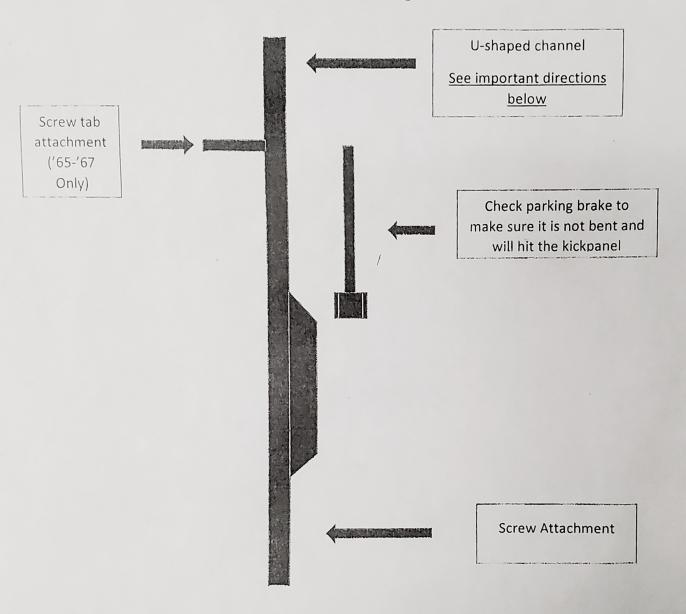
Driver side speaker only clears emergency brake pedal, if kickpanel is installed inside all carpeting, etc. and retaining screw is utilized (forward lower side) on '64 only. The top of the U-shaped channel must be trimmed to match the end of the existing trim on the vehicle. In some vehicles an additional attachment screw may be necessary to pull in kickpanel for brake pedal clearance
