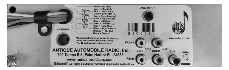
The ANTENNA jack is located above the wiring harness exit. It will accept your original antenna plug.
