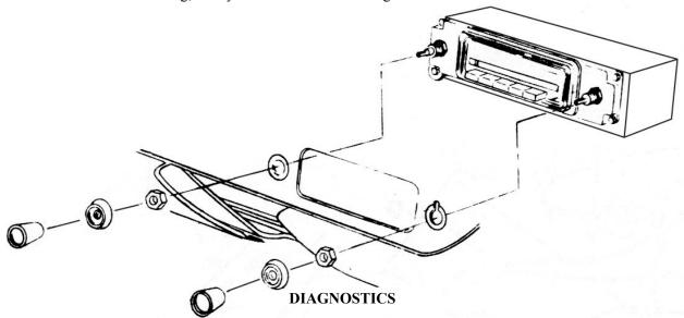
**No Sound:** Check for a good fuse with proper rating. When the radio is turned on, the orange wire should have 12 volts present. Radio will mute when no station is received. Make sure antenna is plugged into the proper jack. If an option is plugged in, make sure it's not on. Before installation make sure the switch on the back of the radio is set for the correct speaker option and country.
