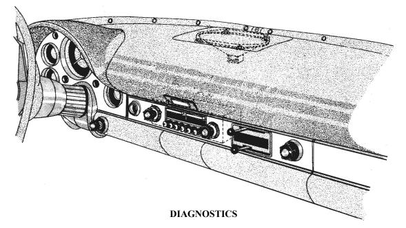
**No Sound:** Check for a good fuse with proper rating. When the radio is turned on, the orange wire should have 12 volts present. Radio will mute when no station is received. Make sure antenna is plugged into the proper jack. If an option is plugged in, make sure it's not on. Before installation make sure the switch on the back of the radio is set for the correct speaker option and country.
