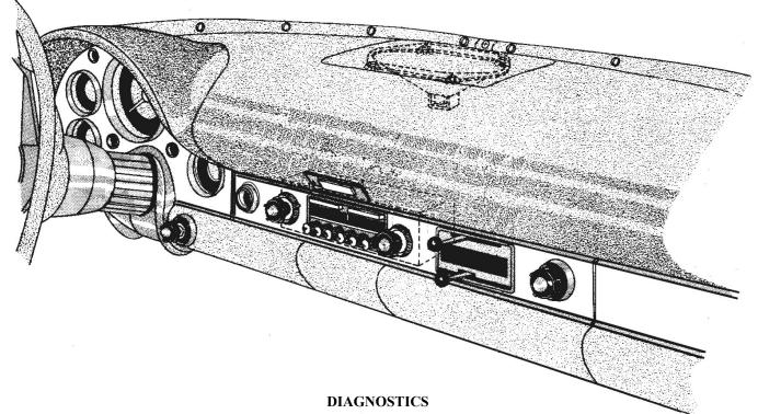
**No Sound:** Check for a good fuse with proper rating. When the radio is turned on, the orange wire should have 12 volts present. Radio will mute when no station is received. Make sure antenna is plugged into the proper jack. If an option is plugged in, make sure it's not on. Before installation make sure the switch on the back of the radio is set for the correct speaker option and country.
