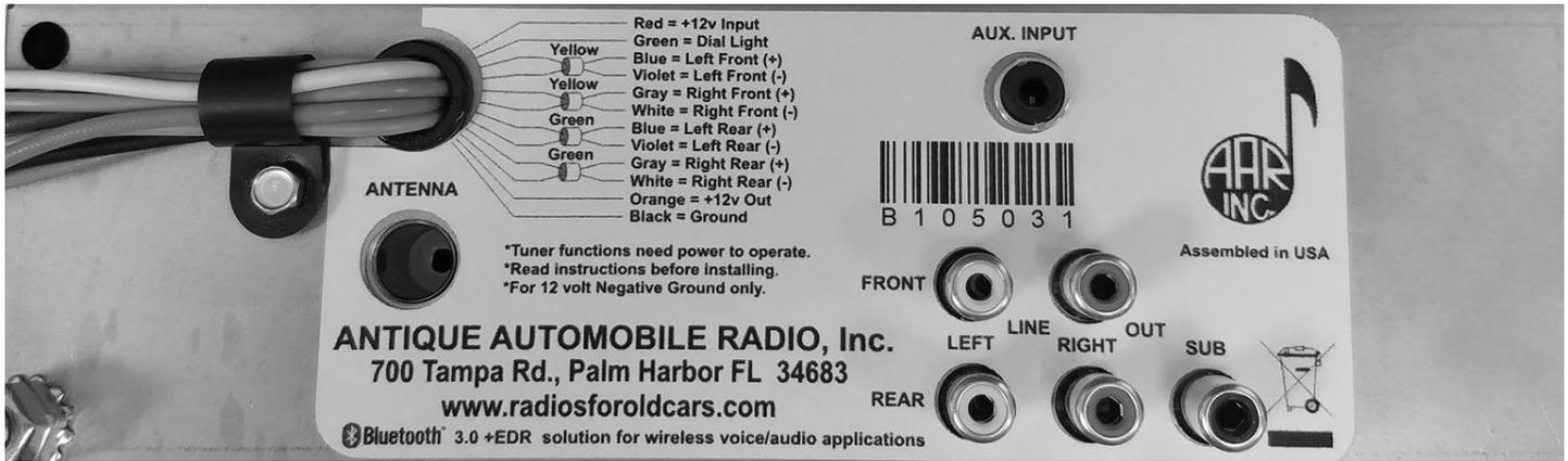
The **ANTENNA** jack is located beneath the wiring harness exit. It will accept your original antenna plug.
