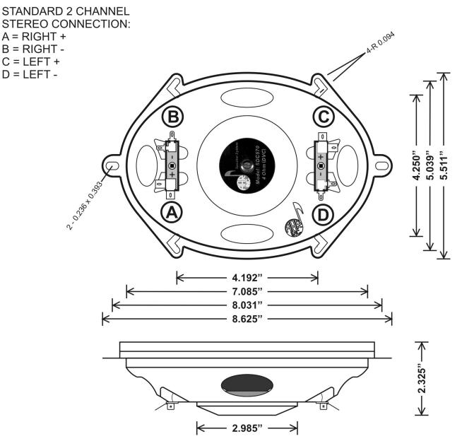
TO REPLACE A SINGLE ORIGINAL 8 OR 10 OHM (MONO) SPEAKER: A = SPEAKER OUT + B CONNECTS TO C D = SPEAKER OUT - OR GROUND IF SINGLE WIRE SPEAKER.
