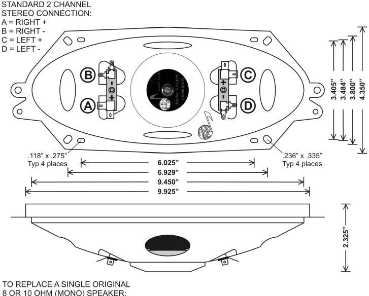
8 OR 10 OHM (MONO) SPEAKER: A = SPEAKER OUT + B CONNECTS TO C D = SPEAKER OUT - OR GROUND IF SINGLE WIRE SPEAKER.
